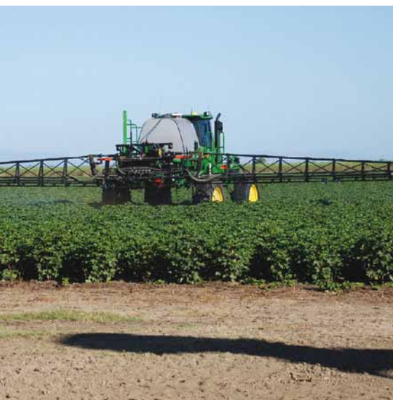
Long spray booms need to be factored in to your safe distances.
